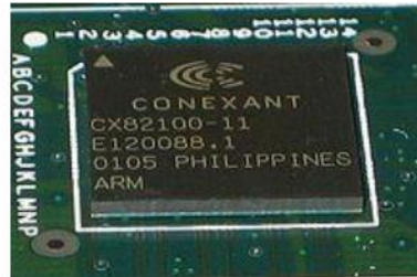
Advanced RISC Machine (ARM) Microprocessor developed by Conexant Computers
